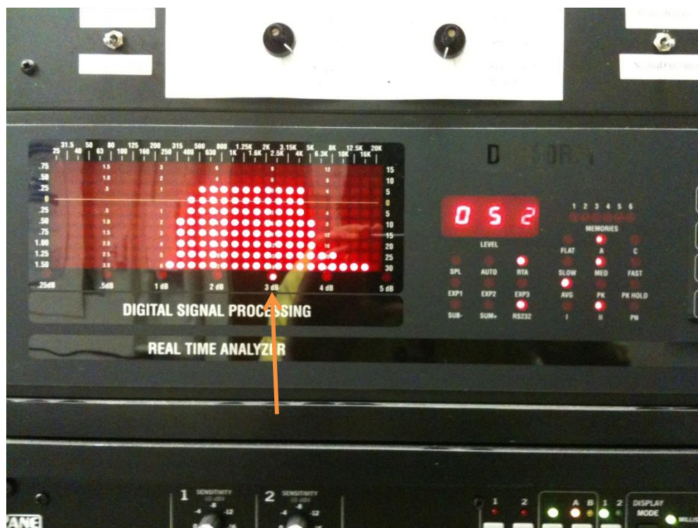
Figure D-3. Real time spectrum analysis of pink noise in Chamber 2.
